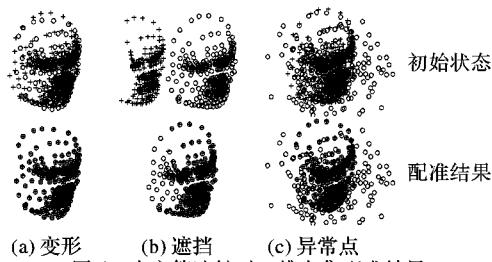
Fig. 5 Registration results of the proposed algorithm for 3D point sets
